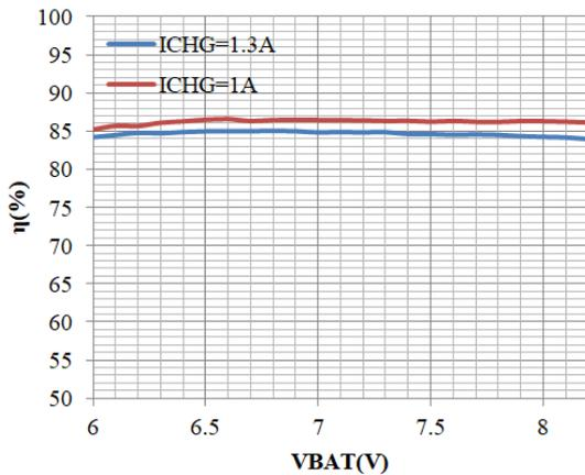
VBATT VS.  $\eta$  (VIN=5V)
